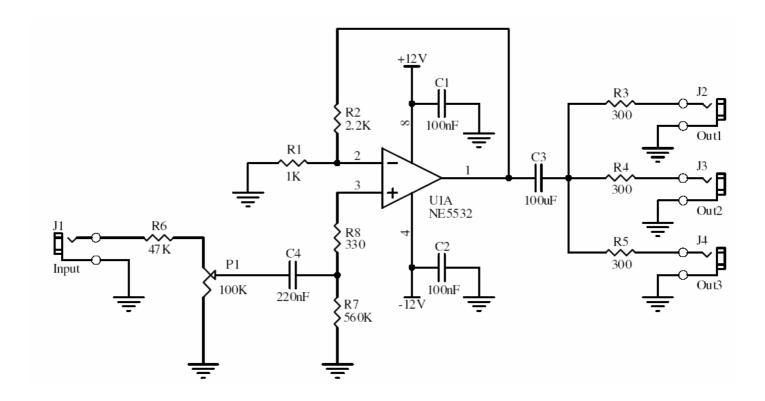
This circuit is suitable to amplify and distribute the audio signals. The input audio signal is applied to the J1 and after passing through the P1, It is buffered and amplified by the U1 prepared to redistribute. It has 3 output to drive 3 audio lines with 300 ohms impedance.
